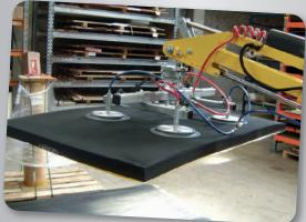
The SL 380 Midi is fitted for window and glass installation as standard, but can be supplied with a special device for lifting, e.g. heavy fire doors and gates.
