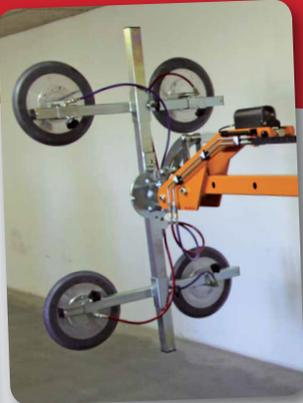
The yoke allows multidirectional movement.
