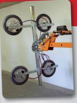
The yoke allows multidirectional movement.
