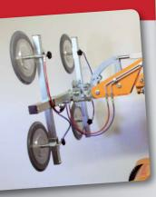
The vacuum system is separated into two circuits (separate blue and red hoses) for the highest level of security.
